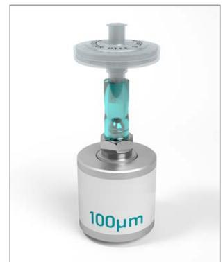
All AtmoCheck TPC units are calibrated with certified hole sizes to make sure that the leak test gives you a high accurate and proper result. Hole sizes 0.5 – 5 µm on request
