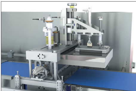
Long dwell transversal jaws with pressure pad
